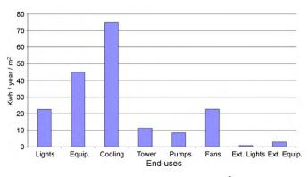
Fig. 5. Electrical end-uses in kWh/year/m<sup>2</sup>.
